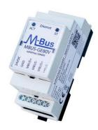
Our MBUS-GE20V and MBUS-GE80V are two level converters for remote applications. They can handle up to 20 or 80 unit loads and are translating the serial data into data packets sent via Ethernet. The IP network allows having the remote device on-site or far-off. A simple TCP socket (or optionally a virtual COM port; we recommend the driver from company Eltima) on the data terminal end is used for transparent M-Bus communication over Ethernet.
